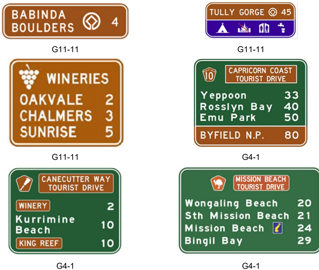
Figure 5.3.5 – Examples of reassurance tourist signs and direction reassurance signs with tourist patch
