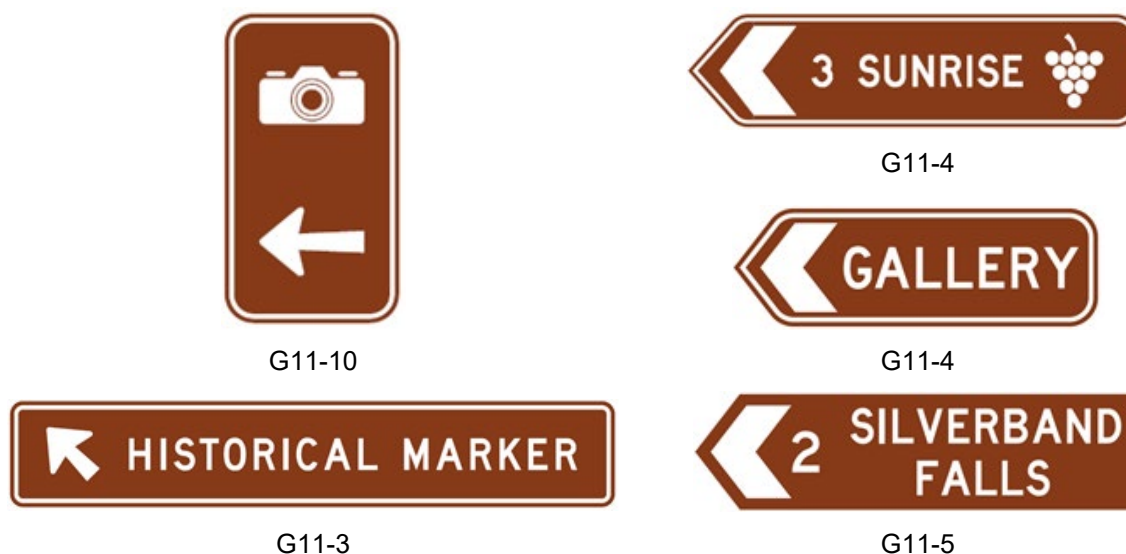
Figure 5.3.6 – Examples of position signs
