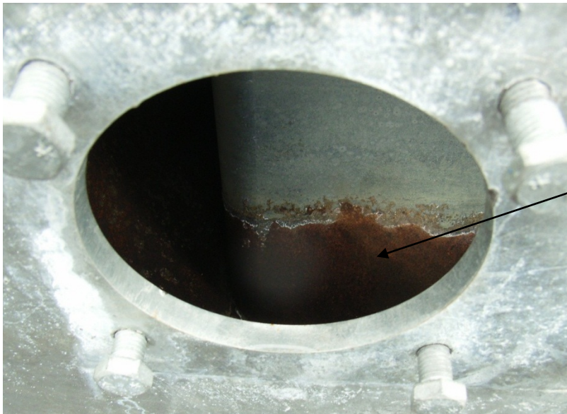
Figure 37 – Close up view of the corrosion
