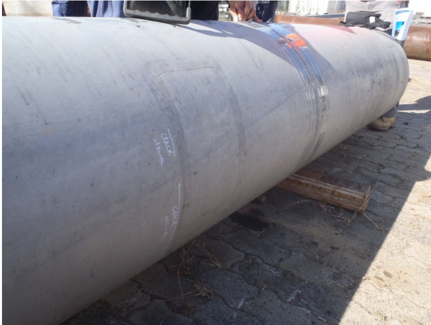
Figure 48 – View of the visual cracks in the butt weld on the back side of the column member
