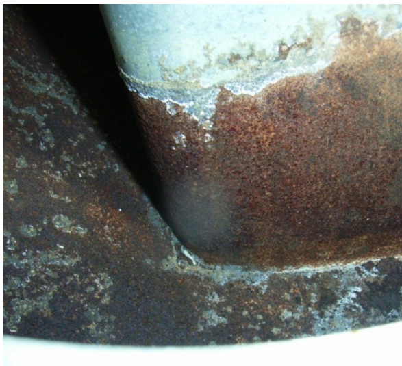
Figure 38 – Corrosion leaching out of vent hole
