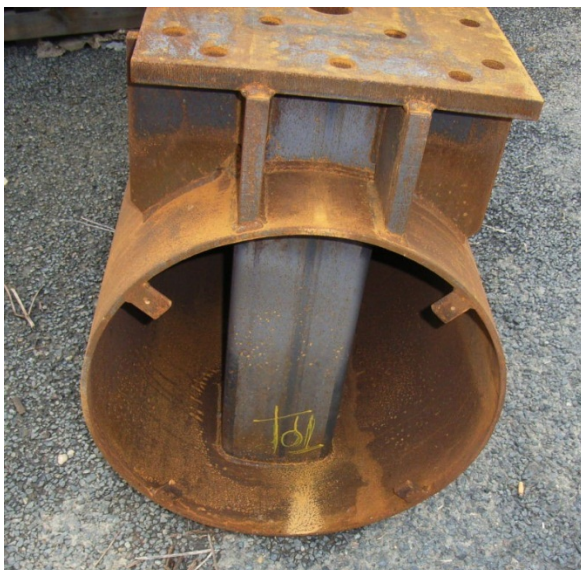
Figure 45 – One way to provide adequate venting is to bolt on the cap plate
