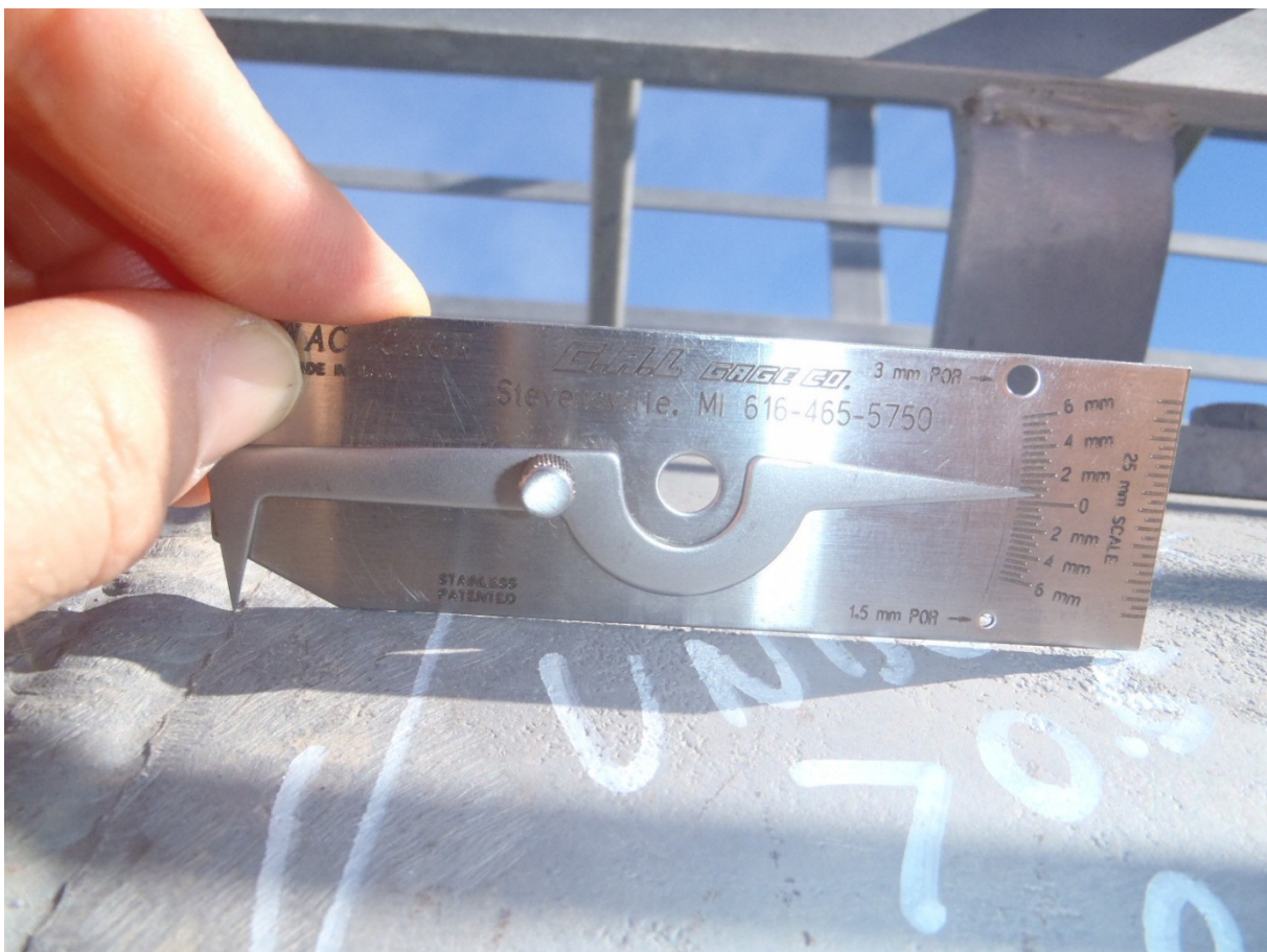
Figure 52 – View of the level of undercut in the butt weld
