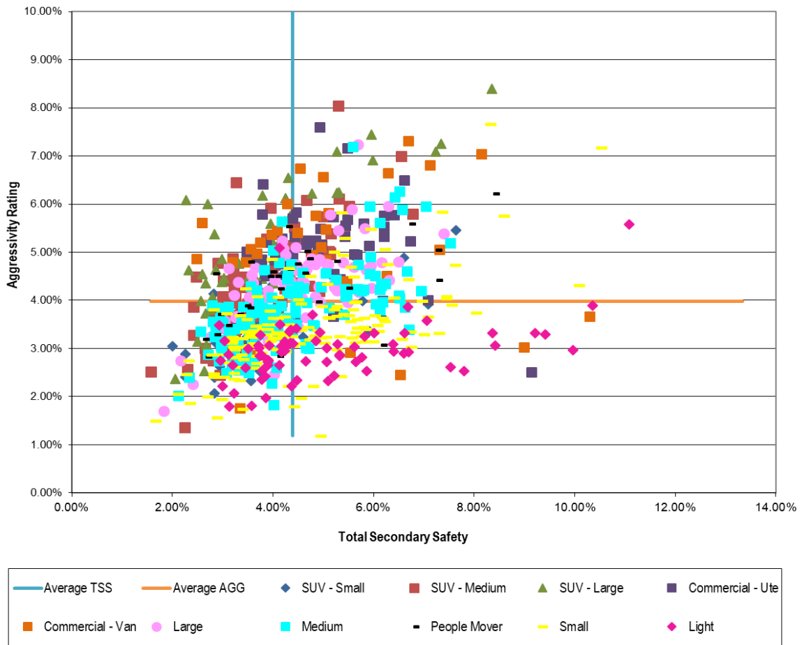
Figure 13: Aggressivity vs. Total Secondary Safety
