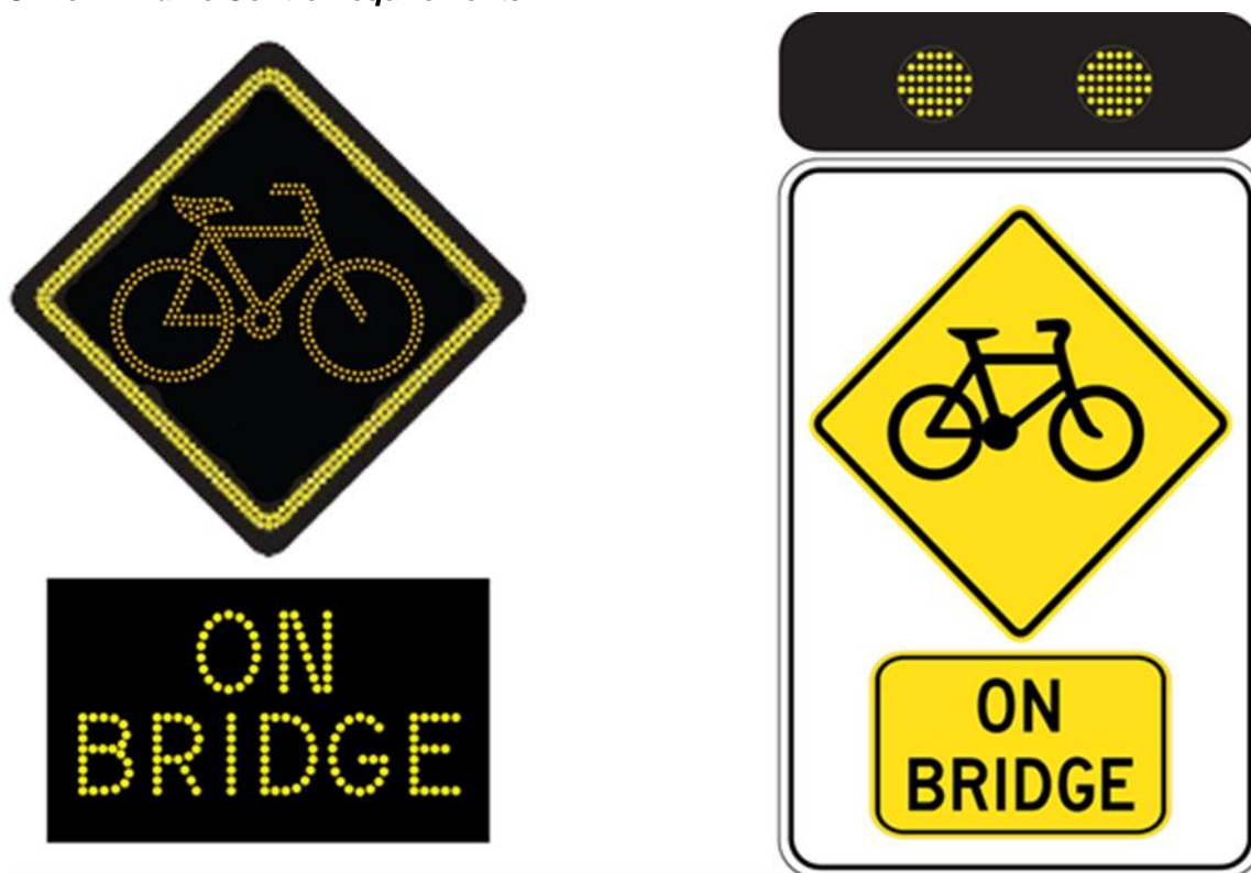
Figure 6(a) – Examples of bicycle activated warning signs that replicate Queensland Manual of Uniform Traffic Control requirements
